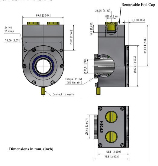
Plastic screw plugs are provided for cable outlet protection during shipping and storage. These plastic plugs must be replaced by an EX d certified cable gland or blind plug prior to use.
